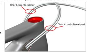
Please be aware, to prevent damage to the frame and cables there should be minimum cable clearance between the bottom of the bottom bracket and the cables.
