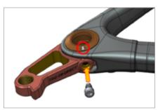
Make sure the location arrow is pointing to the lower bolt hole; insert the bolt (Max torque 1.5 N/M)
