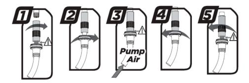
Please note that air will flow into the hose and indicator when counterchecking the air pressure, this will give the appearance that the shock has less air pressure then it was setup, your shock may need to be adjusted once this action is made.
