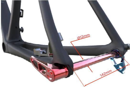
Hinterradachse Solace Disc SCOTT
